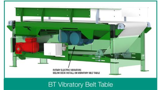
Most of the vibratory equipment manufactured by Cleveland Vibrator uses two rotary electric vibrators to produce linear vibration. Vibratory tables, vibratory grid tables, electromechanical screeners and electromechanical feeders are all designed for the vibrators to counter rotate.
